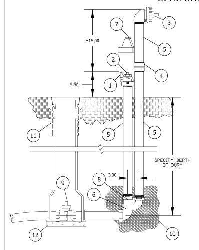
MAINGUARD #77 BLOW-OFF HYDRANT SHALL BE SELF-DRAINING, NON-FREEZING TYPE WITH A
